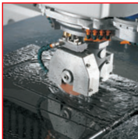
Lucidatura sgocciolatoi. Water slots polishing.
